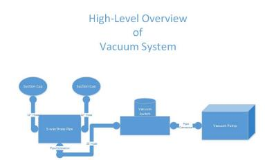
Fig. 23: Final High Level Overview of Vacuum System [20].
