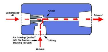
Fig. 3: Working Process of a Vacuum gripper [3].
