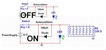
Fig. 26: Solenoid Valve Circuit [23].
