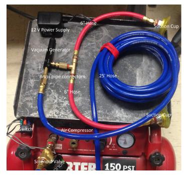
Fig. 20: Vacuum System Components [18].
