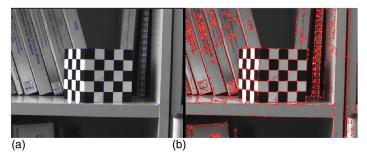
Fig. 1: Example of Edge Detection. [1]
