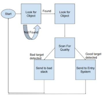
Fig. 24: High Level view of the Vision System [21].
