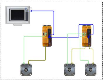
Fig. 25: Overview of Motion Control System [22].
