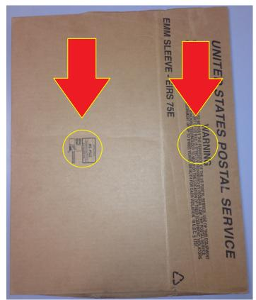
Fig. 15: Marks left by suction cups. Note: not to scale & the color yellow was used to show a clear distinction [13].
