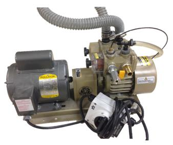
Fig. 21: Vacuum System Pump [19].
